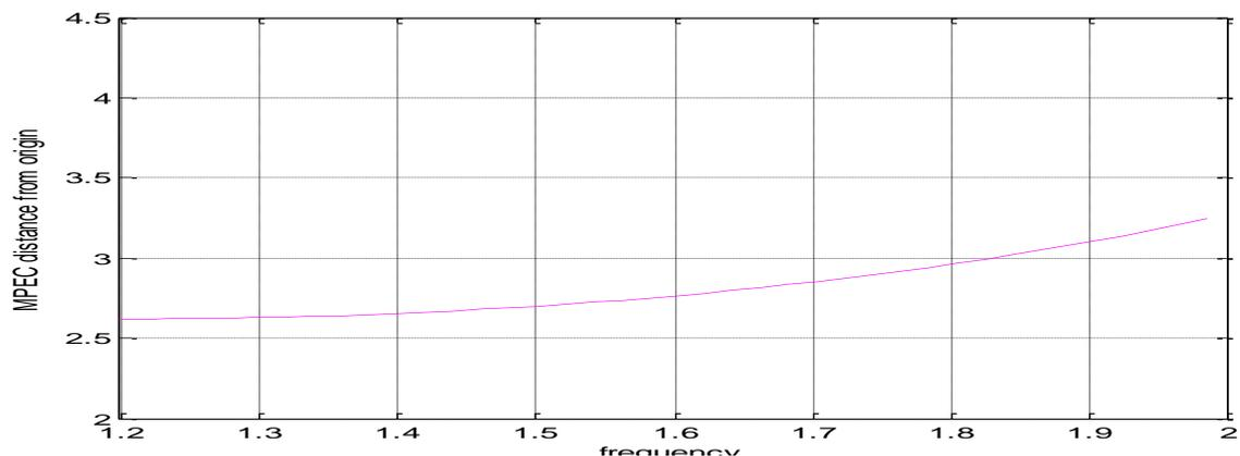
Figure 4. MEPC displacement of horn antenna with frequency
