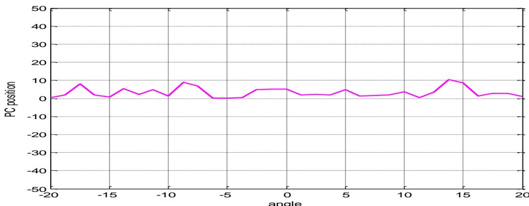
Fig. 2. PC variation of patch antenna beam with angle at 1.4 GHz
