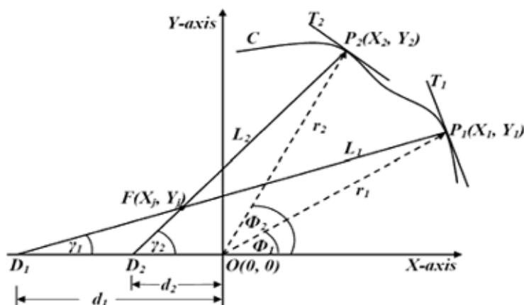
Figure.1. Geometry for analysis of phase centre
