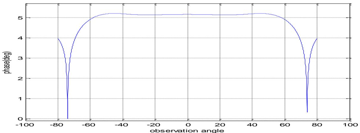
Fig. 5. Phase pattern of horn antenna at 1.5 GHz
