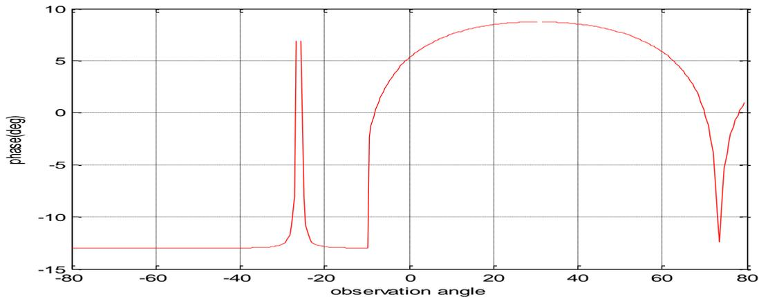
Figure 3. Phase radiation pattern of GNSS patch antenna at 1.2 GHz
